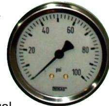
**Differential Pressure** or **Delta Pressure** represented by the symbol  $\Delta$  is equal to the Inlet Pressure minus the Outlet Pressure when the RO is running.
