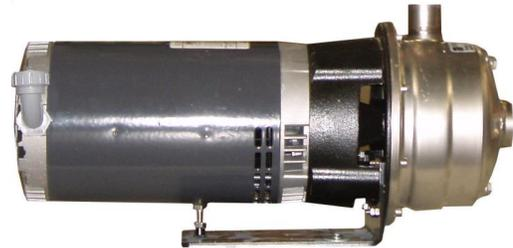
The pump starts automatically when the RO starts or when any of the pre-treatment components that backwash or regenerate start that cycle. This pump is designed for boosting water pressure to the water treatment system, and includes a variable frequency drive (VFD) to speed-up or slow-down the city booster pump as needed.
