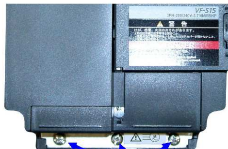
New Model VFD Three grounding posts
