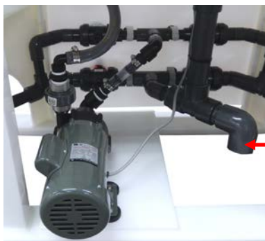
Bicarb Unit, Back View, Denoting Drain Connection
